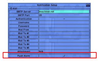
In Alarm Setup, press  $\blacktriangle \lor \blacktriangleleft \blacktriangleright$  to change the highlighted option to Notification, and then press ENTER to enable the notification for the designated alarm.
